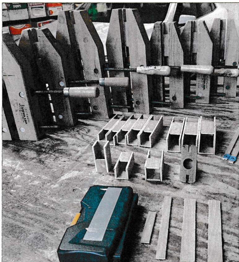
Constructing nozzles. Note the clamped nozzles and the ones in the middle are double ended; these will be cut into two
