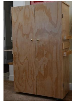
Photo 10. The 49-note Manischewitz organ with the doors on it. Note the handles on the middle of each end the upper ones of which are used to lift the top off the bottom once the doors are lifted off
